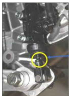
Rear master cylinder push rod & lock nut with permanent color marking
